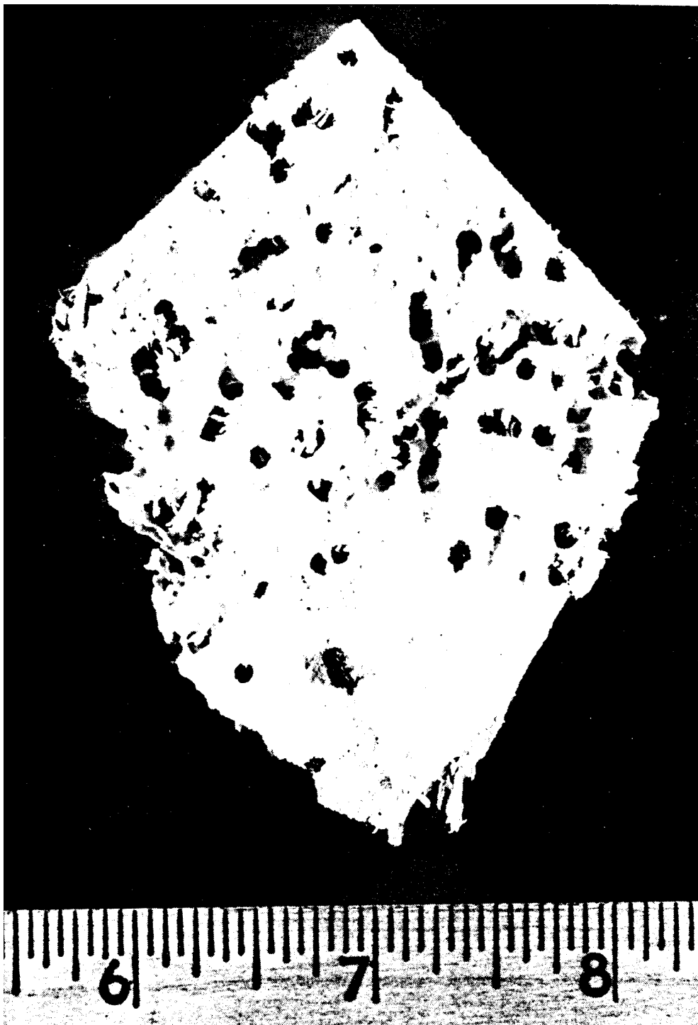
FIGURE 4-23 Bostrichid Damage in Hardwood
